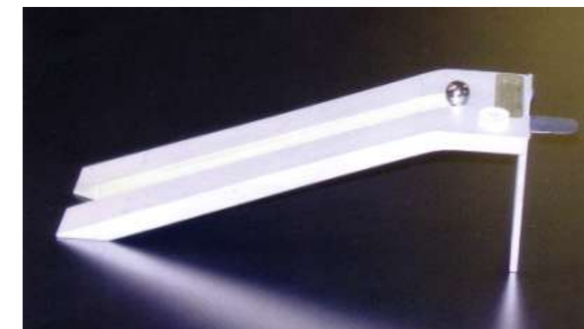
Fig. 4: Rolling ball tack
