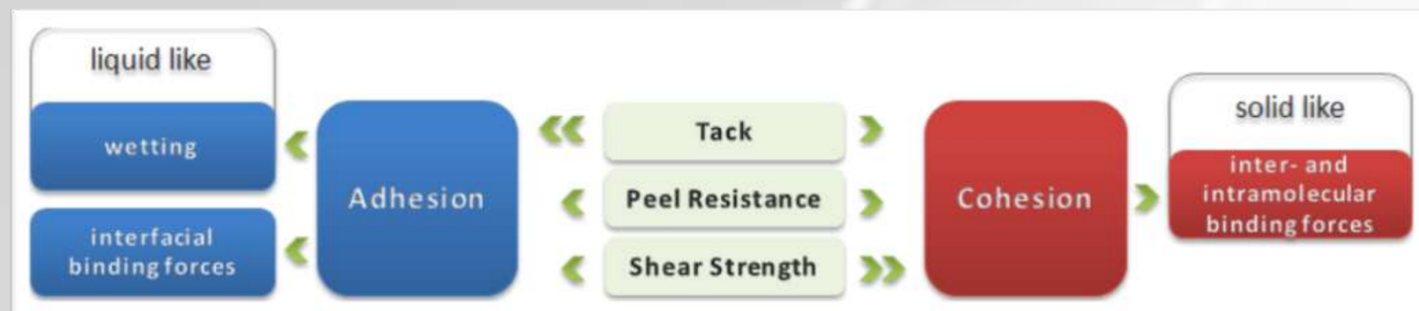
Fig. 1: Characteristics of a pressure sensitive adhesive
