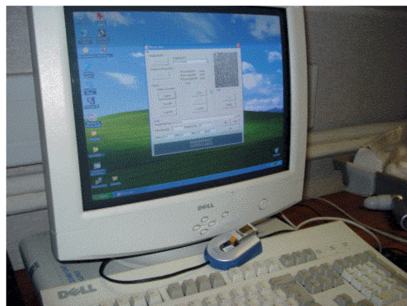
Figure 1. The hand-held probe based on FingerPrint Cards area sensor development kit.
